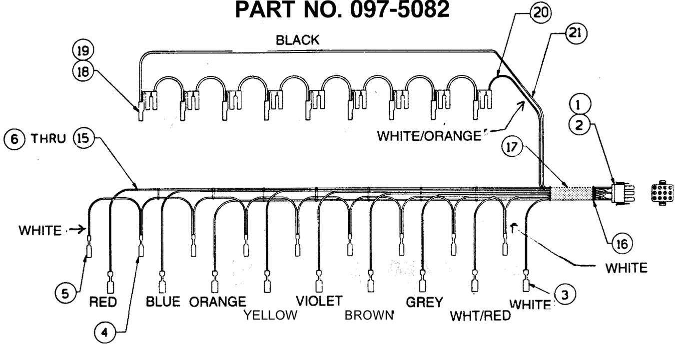
NOTE: THIS HARNESS IS LOCATED ON THE COLD FOOD DOOR AND CONNECTS TO THE DOOR SOLENOID INTERCONNECT HARNESS.
