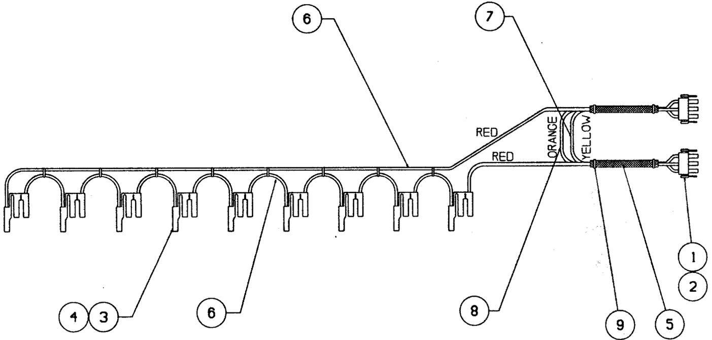
NOTE: THIS HARNESS IS LOCATED IN THE COLD FOOD DOOR ASSEMBLY AND CONNECTS TO THE SHOPPER MOTOR FEED HARNESS AND SHOPPER INTERCONNECT HARNESS.
