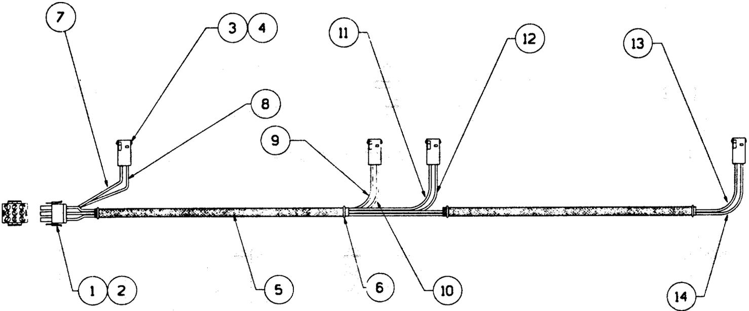
NOTE: THIS HARNESS CONNECTS TO LOWER LAMP SOCKET ASSEMBLY, UPPER LAMP SOCKET ASSEMBLY AND LAMP INTERCONNECT HARNESS.
