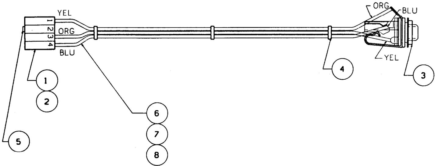
NOTE: THIS HARNESS IS LOCATED ON THE SERVICE DOOR ASSEMBLY AND CONNECTS TO THE CONTROLLER, ALSO MOUNTED ON THE SERVICE DOOR.
