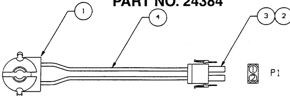
NOTE: THIS HARNESS ASSEMBLY IS LOCATED IN THE COLD FOOD COMPARTMENT LOWER UPPER GUARD ASSEMBLY.
